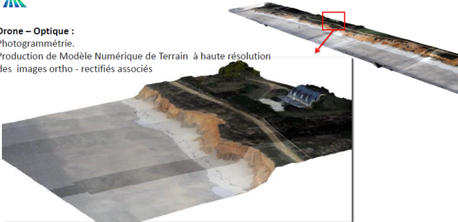
DEM and ortho-photo on Pesnestin Cliff, 2 km-long, resolution 2 cm (2012)
