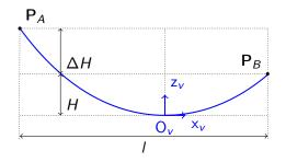
Figure: Catenary of length *L* hanging between  $P_A$  and  $P_B$ .
