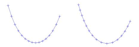
Figure: Normal discretization. Figure: Curvilinear discretization.
