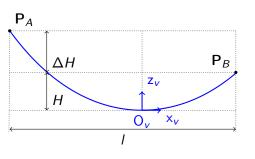
Figure: Catenary of length *L* hanging between  $\mathbf{P}_A$  and  $\mathbf{P}_B$ .
