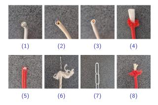
Figure: Pictures of the different cables used in the experiments: (1) coaxial cable; (2) four pairs ethernet cable; (3) two pairs ethernet cable; (4) floating rope; (5) rope; (6) weighted rope; (7) steel chain; (8) elastic rope.
