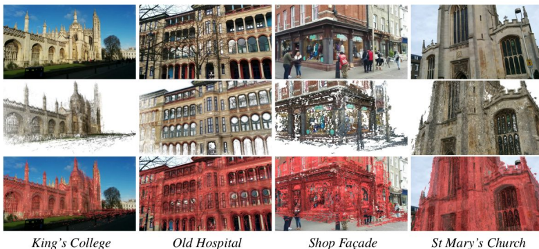
Figure 1: PoseNet: Convolutional neural network monocular camera relocalization. Relocalization results for an input image (top), the predicted camera pose of a visual reconstruction (middle), shown again overlaid in red on the original image (bottom). Our system relocalizes to within approximately 2m and 6^\circ for large outdoor scenes spanning 50,000m^2 . For an online demonstration, please see our project webpage: mi.eng.cam.ac.uk/projects/relocalisation/
