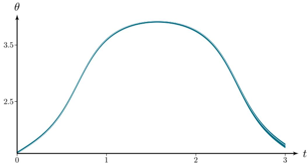
The tube  $[x_3](\cdot)$  of feasible headings. The actual but unknown truth is plotted in white and guaranteed to be enclosed in the computed  $[x_3](\cdot)$ .
