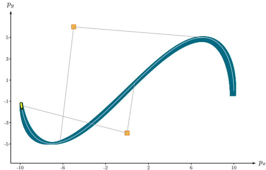
Set  $[x](\cdot)$  of feasible states projected in two dimensions. The unknown planar trajectory remains enclosed in the tube.
