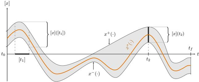
Fig. 2. A tube  $[x](\cdot)$ , interval of two functions  $[x^-(\cdot), x^+(\cdot)]$ , enclosing a random signal  $x^*(\cdot)$ .
