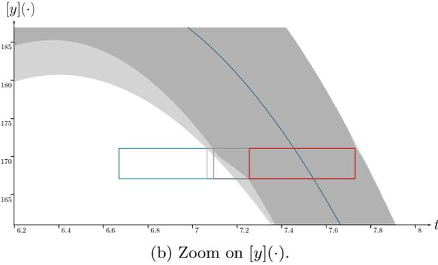
Fig. 11. Tube  $[y](\cdot)$  representing the reliable prevision of the distances between the boat and the beacon (so-called *ephemeris*).  $[y](\cdot)$  is submitted to a set of measurements pictured by blue boxes, before their final contraction in red. This demonstrates the contraction of strong time uncertainties by  $C_{\text{eval}}$  thanks to the knowledge provided by the tube itself.
