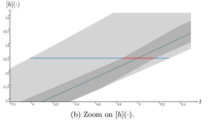
Fig. 12. Tube  $[h](\cdot)$  representing the clock drift. For a given time  $\tau_i$ ,  $[h]^{-1}(\tau_i)$  provides an enclosure  $[t_i]$  of the time reference  $t_i$ . When  $[t_i]$  is contracted by means of ephemeris  $[y](\cdot)$  and  $C_{\text{eval}}$  (see Figure 11), the information can be propagated back to  $[h](\cdot)$ . The tube's contracted part is pictured in light gray while the real drift expressed by Eq. (16) is plotted in blue.
