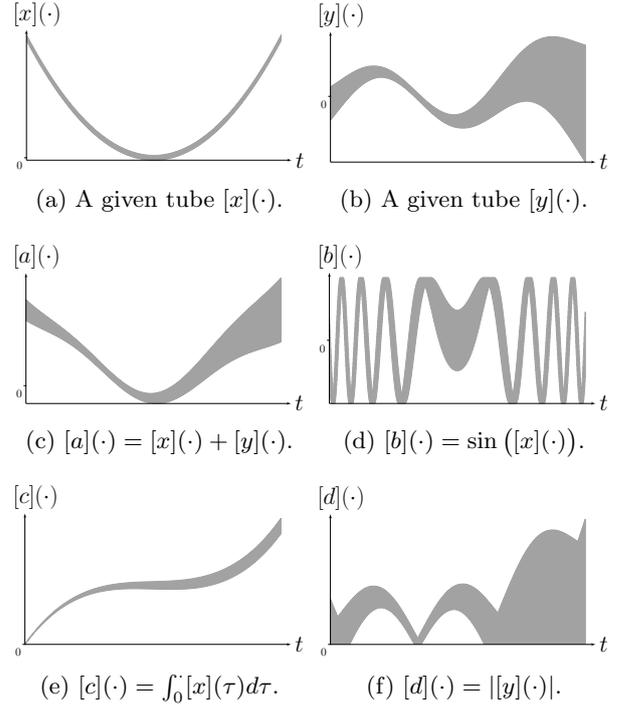
Fig. 3. Tube arithmetics. Note that the vertical scales of these figures vary for full display.
