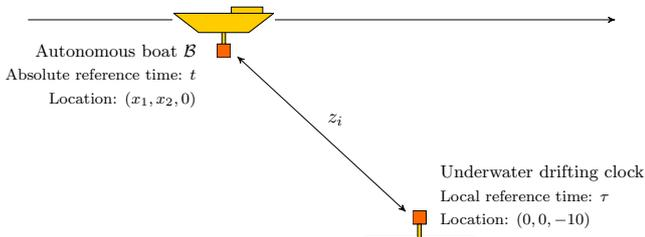
Fig. 10. Illustrating the problem of a drifting clock corrected by ephemerides provided by an autonomous boat  $\mathcal{B}$ . The beacon holding the clock receives distance measurements from the boat once in a while.
