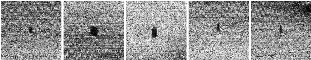
Figure 1: Different underwater rocks perceived with one side-scan sonar. These observations are view-point dependent and the sonar images are noisy, which makes it difficult to distinguish one rock from another only from image processing. These sonar images have been collected by the *Daurade* robot (DGA-TN, Shom, Brest) equipped with a Klein 5000 lateral sonar.
